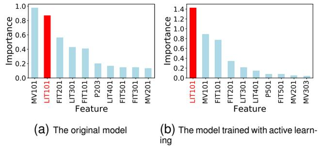
Fig. 6. The feature importance of the LSTM model that predicts the evolution of MV101 which is trained (a) normally and (b) with active learning techniques
