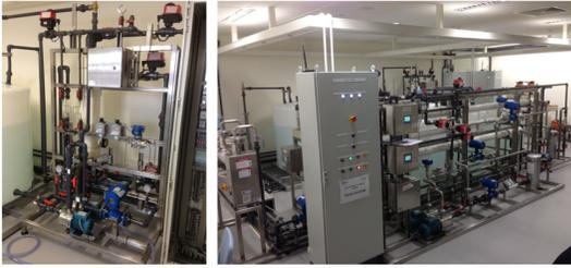
Fig. 1. The Secure Water Treatment (SWaT) testbed
