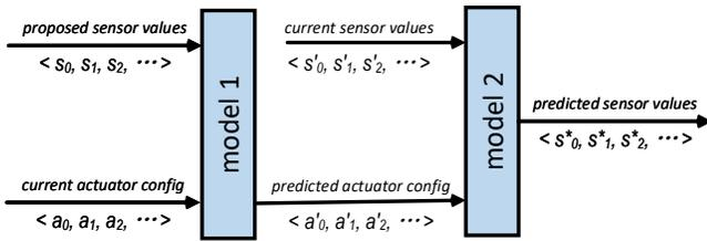
Fig. 3. Inputs/outputs of the learnt models
