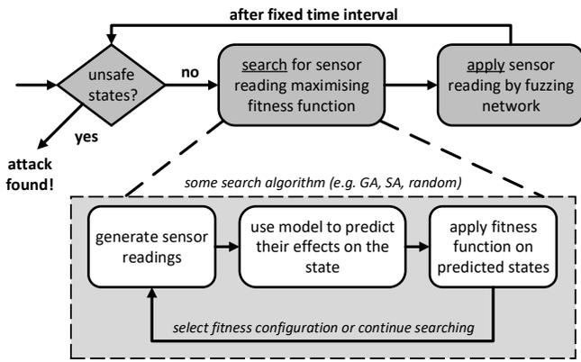
Fig. 4. Overview of our ML-guided sensor fuzzing (details of any particular search algorithm are omitted here)
