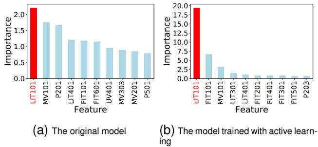
Fig. 5. The feature importance of the SVC model that predicts the evolution of MV101 which is trained (a) normally and (b) with active learning techniques
